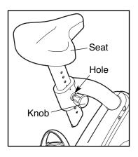
slide the seat post upward or downward, and align one of the adjustment holes in the seat post with the indicated hole in the seat frame. Then, release the seat knob into the seat frame and the seat post, and turn the knob clockwise until it is tight. Make sure that the seat knob is inserted through one of the adjustment holes in the seat post.
